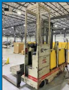
6,600 Lb. Kalmar Model EFY-30/14/40-FL Electric Side Loader
